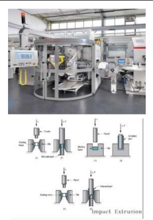
Impact extrusion is a manufacturing process similar to drawing by which products with metal slugs are made. The snail is pressed very fast with a punch into the die or mold.
